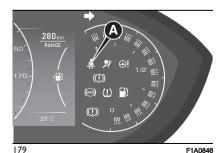
As soon as a speed threshold of 20 km/h is reached, with driver side seat belt or the passenger side seat belt (with occupant seated) unfastened, an acoustic warning is activated simultaneously with warning light flashing for about 105 seconds.
