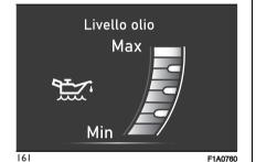
If the oil level is lower than the minimum required value, the display shows a dedicated message indicating minimum engine oil level and the need for a topup.
