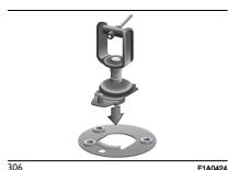
☐ tighten the knob onto the screw to secure the bracket fig. 307;
