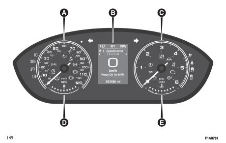
A. Speedometer B. Multifunction display C. Tachometer D. Fuel level gauge E. Engine coolant temperature gauge WARNING The illumination of the instrument panel graphics may vary according to version.
