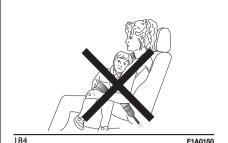
Each seat belt must be used by only one person. Never travel with a child sitting on the passenger's lap and a single belt to protect them both fig. 184. In general, do not place any objects between the person and the belt.
